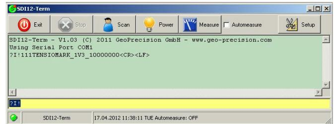
The most important SDI12 commands (letters a and b are for SDI addresses (0..9, a-z, A-Z, the question mark stands for „unknown“ and works only, if only one sensor is connected to the SDI 12 bus, if several sensors are connected, it can not be used.):
