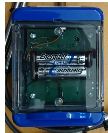
String-Box Higher battery capacity and extended wireless-range (external antenna).
